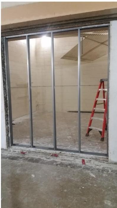
Figure 2 – Framing members installed in test aperture
